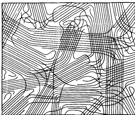
FIG. 3. Fringed micelle model of crystallite structure.
